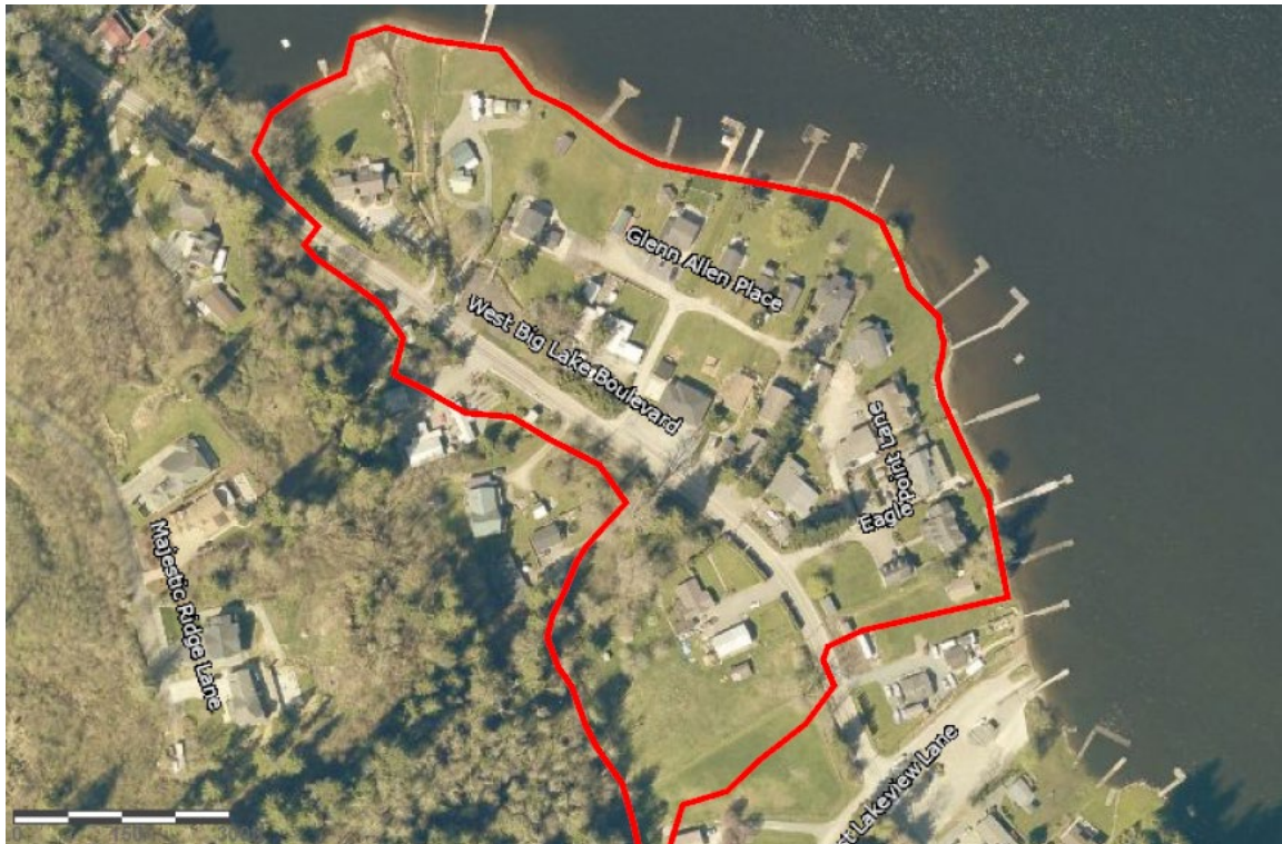
Figure 18. Estimated extent of flooded area from review of drone footage.
